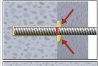
Annular gap between reinforcing bar and base material must be completely filled with mortar. Otherwise, the installation must be repeated starting from step 8 before the maximum working time  $t_{work}$  has expired.
